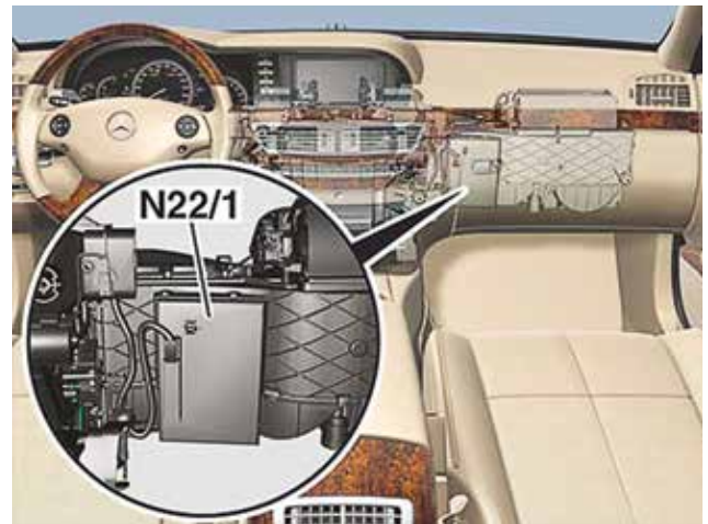
The ACC (NC22/1) combines input from the dash controls with feedback from a variety of onboard sensors, and applies algorithms to make A/C function decisions that help Mercedes-Benz vehicles maintain their fuel-sipping attributes.
