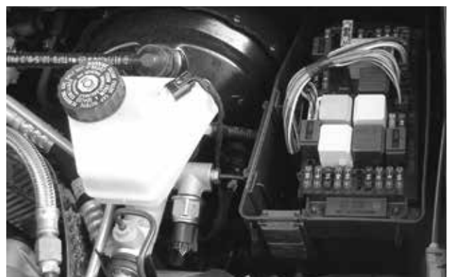
The driver's-side SAM generates a pulse width modulated (PWM) signal to tell the compressor control valve what refrigerant displacement level is needed for conditions.
