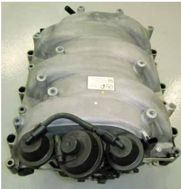
On this M272 intake manifold the vacuum actuator for the actuation of the tumble/swirl flaps is located between those for the variable runner flaps.
