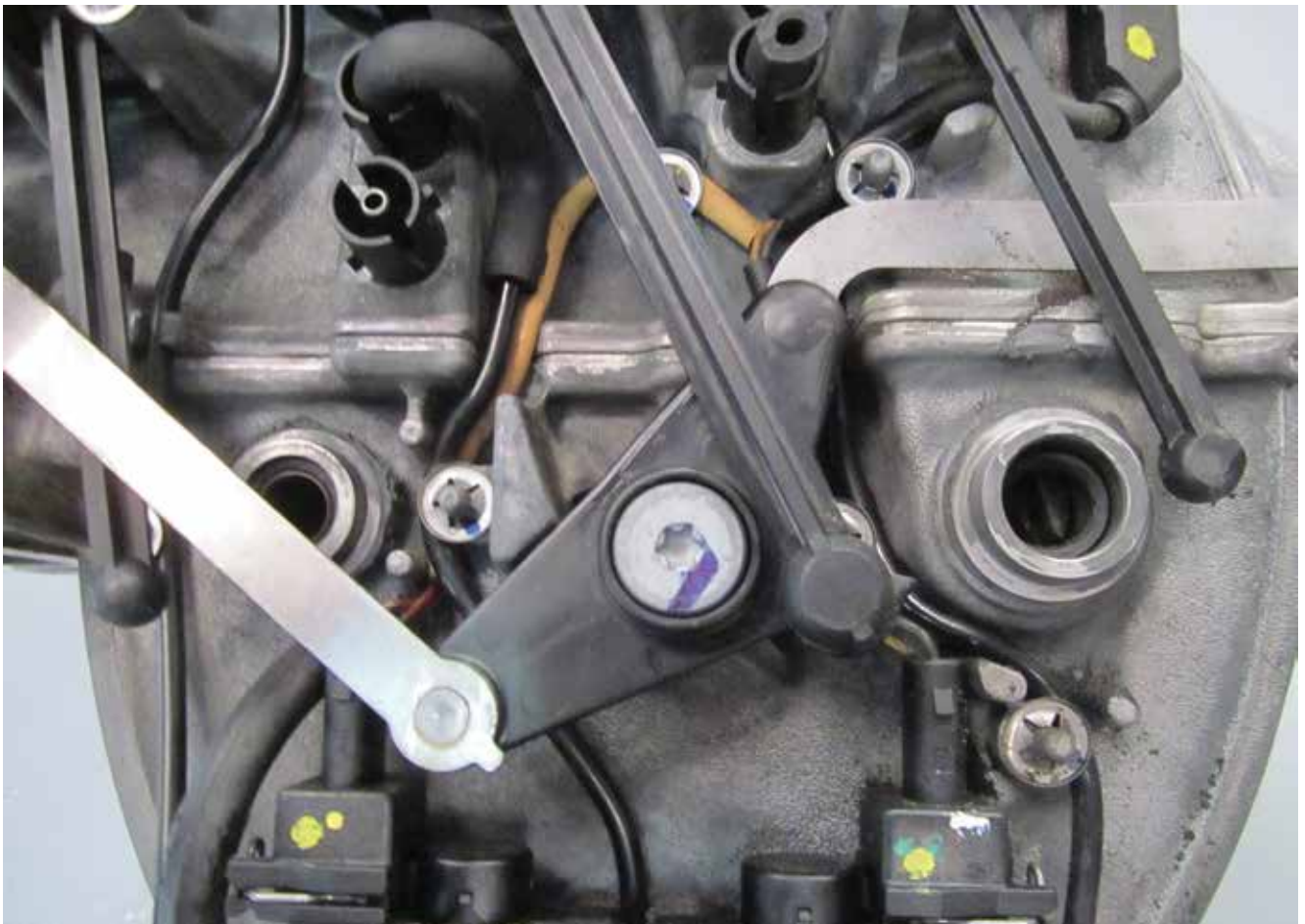
This M272 engine was neglected to the point that the flaps stuck and broke, as did the vacuum actuator rods. Plastic from the flaps was ingested into the cylinders, bending valves.
