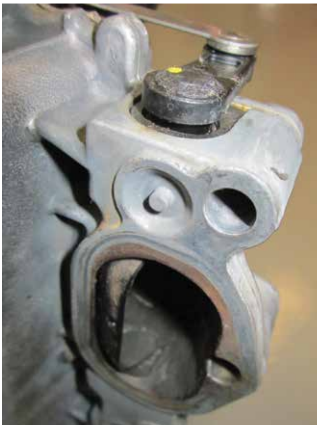
The tumble/swirl flaps are located directly upstream of the manifold runner/cylinder head intake port interface.
