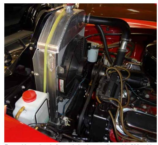
Even with an electric fan and aluminum radiator this 500 cubic inch Cadillac engine in this '41 Caddy tended to overheat every time the weather got warm.
