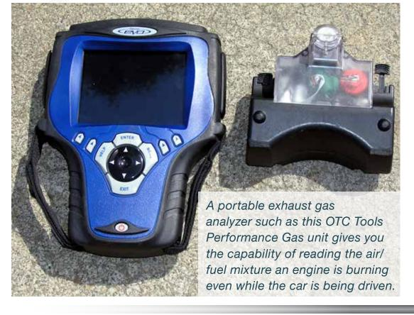
power circuit should also be checked to be sure it's adequate for high-load operating conditions. Most vintage engines use a power mixture of 6.6% CO, or a 12:1 air/fuel mixture, while an engine with more modern fast-burn cylinder heads may operate best with a 13.2:1 power ratio. If the mixtures are richer than the targets mentioned, the engine may not run too hot, but it may foul spark plugs and the vehicle will not go as far on a gallon of gas as it would if it were properly tuned.
