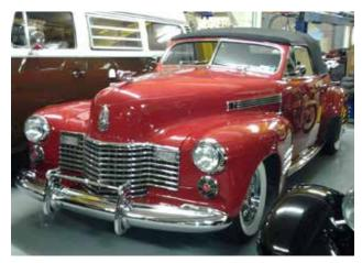
The 500 cubic engine in this 1941 Cadillac now performs very well indeed, and it never overheats. The cures were routing all the air flow through the radiator, and proper tuning.
