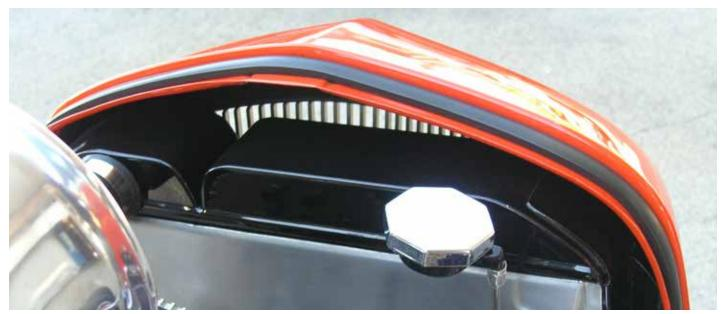
The air gap above the radiator of this supercharged street rod is allowing cool air to flow around the radiator instead of through it.
