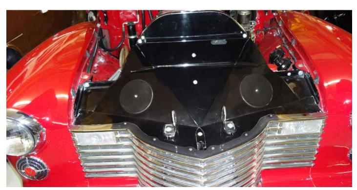
Once the access holes in the radiator supports of this 1941 Cadillac were covered, the engine ran cooler at highway speeds.
