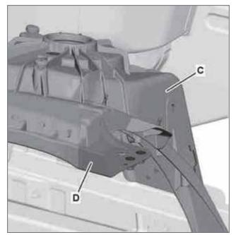
The connecting flange for the front module carrier (D) on the suspension strut tower (C) can be straightened only if the deviation is vertical, i.e., higher or lower than specified, and only if it is off by a minor amount. If the deviation from the measuring point is greater than 10 mm, the suspension strut tower component must be replaced rather than straightened (see "Checklist for damage diagnosis in the event of an accident" in WIS for further details).
