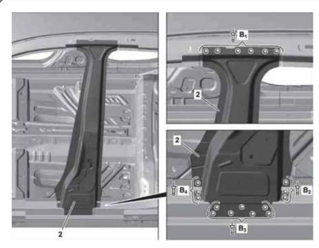
On the GLA 250, the B-Pillar reinforcement is made of Ultra-High-Strength Steel. To replace, fit the new B-Pillar reinforcement (2) in place, drill 6.7 mm rivet holes at areas B1, B2, B3, and B4. Remove the B-Pillar reinforcement, deburr rivet holes on B-Pillar reinforcement (2) on both sides. Remove drilling shavings with wet/dry vacuum, then coat the inside of the riveted joints with zinc dust paint.
