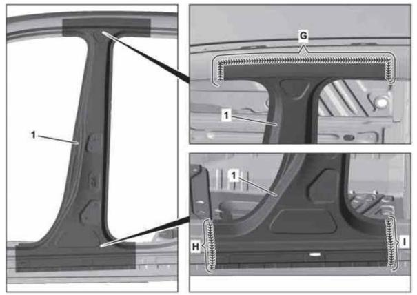
After assembling all B-Pillar components, inert gas weld in areas G, H and I on the outer B-Pillar, allowing each weld to cool before starting the next area. Grind the welds down flat. Solder surfaces in areas G, H, and I with body solder and smooth over.
