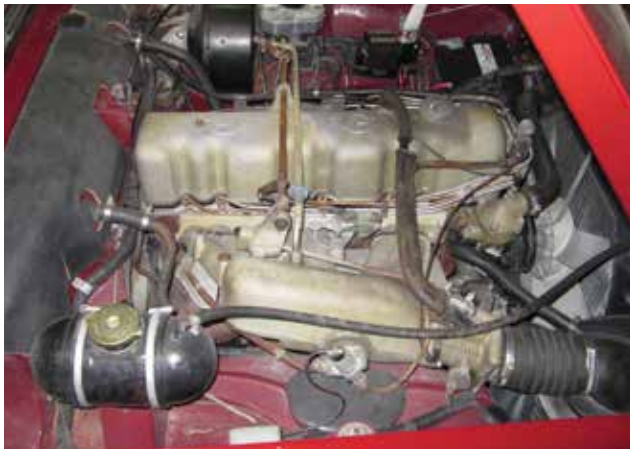
This 1970 Mercedes SL280 engine operated with a fixed fuel curve. These ran normally at between 2 and 6% CO (carbon monoxide) emissions. We have come a long way.
