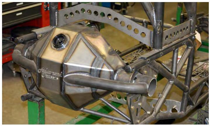
This gives you a good idea of what talent with a welder can get done. This Mini-mod pulling tractor frame is going together with a custom-fabricated rear axle housing.
