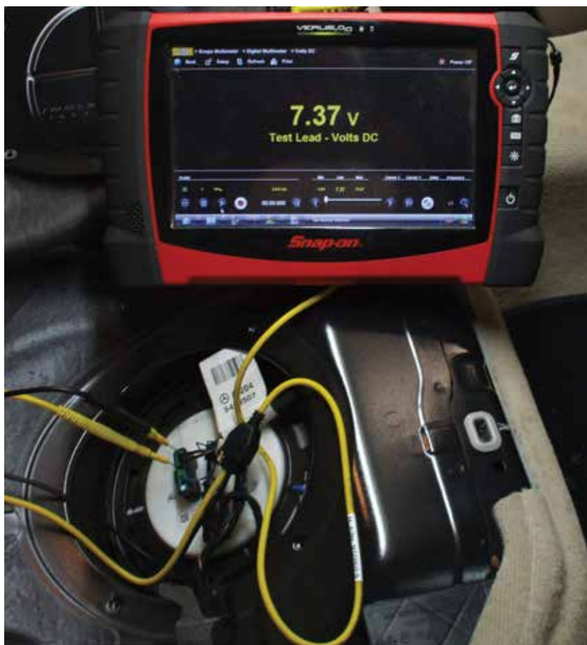
It's not just for fuel injectors anymore. Here's the average voltage of PWM signal to the fuel pump on a Mercedes-Benz W204 chassis C350 as seen on a lab scope.
