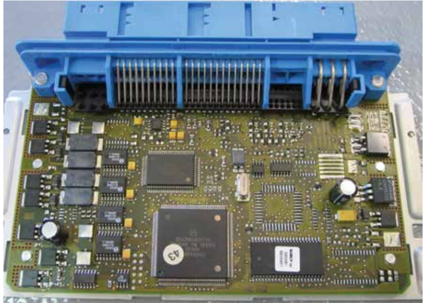
Here's a modern-day ECU with multiple MOSFET PWM relays.
