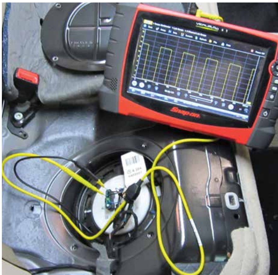
The live data stream for a W204 chassis C350 fuel pump at idle.
