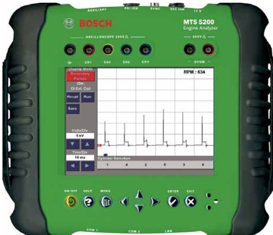
A modern engine analyzer such as this Bosch MTS 5200 offers an ignition scope, cylinder balance, and vacuum per cylinder, all in a hand-held unit.
