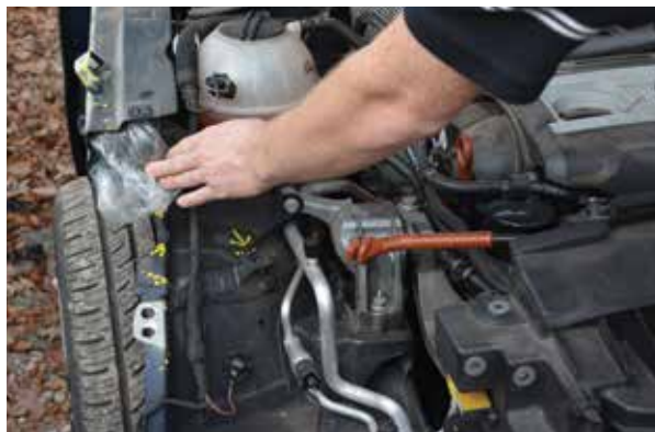
Check your repair information for locations of sound-deadening insulation in the repair area, and replace it if missing or damaged.
