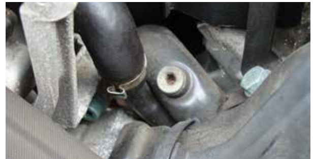
Don't overlook other cooling system bleed points.
