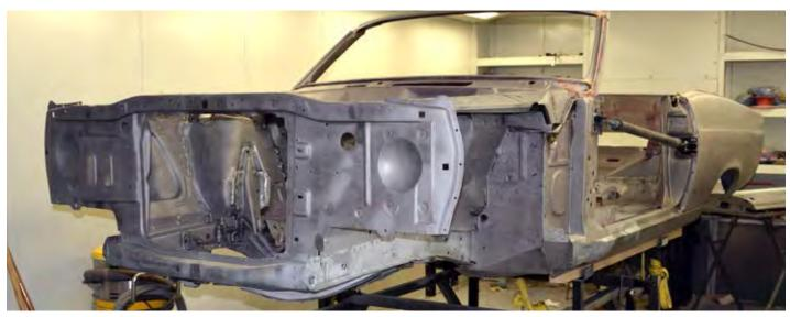
Many paint-removal facilities first bake the parts to cook out old body seam sealer and loosen the paint on the surface. Then they typically attack the residue with plastic blast media and carefully-regulated air pressure to finish it off. Needed repair work aside, it's not going to be paint ready -- it'll still need work with a sander or DA -- but it'll save you a ton of time if you get the big chunks off first.
