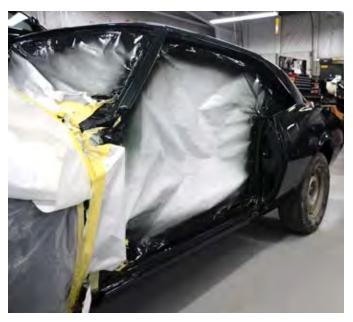
When and where possible, you can combine your cut-in work and the first color coat. It all depends on the project and how much of the car is dismantled. No point in making extra work or shooting overlapping color coats if you don't have to. Paint takes on a different look depending on temperature and humidity, so shooting as much as you can in one session just minimizes having an appearance problem that you'll have to fix.
