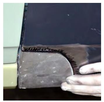
If you have enough damage and access to quality replacement sheet metal, then certainly panel replacement is the better option, but for small areas making your own patch panels is a less-expensive and faster alternative. Equipment like a sheet metal break, a shrinker-stretcher and a power roller make life a little easier, but it's the hands, hand tools, and patience of the artisan that makes it look as if the panel has never been modified after all is said and done.
