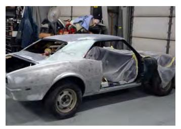
This NOS GM quarter panel is hung, spot welded, and seam-sealed. You can see that the lead seam on the sail panel has been replaced with modern materials. While it looks like a lot of material has been applied, it's very thinly spread, tapering off to nothing, to hide the seam transition.
