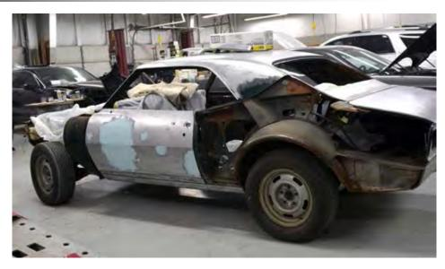
aft. There's a lot of pre-fitting, doublechecking and prep work to do before the panel is welded on, but you can see what the thought process is.
