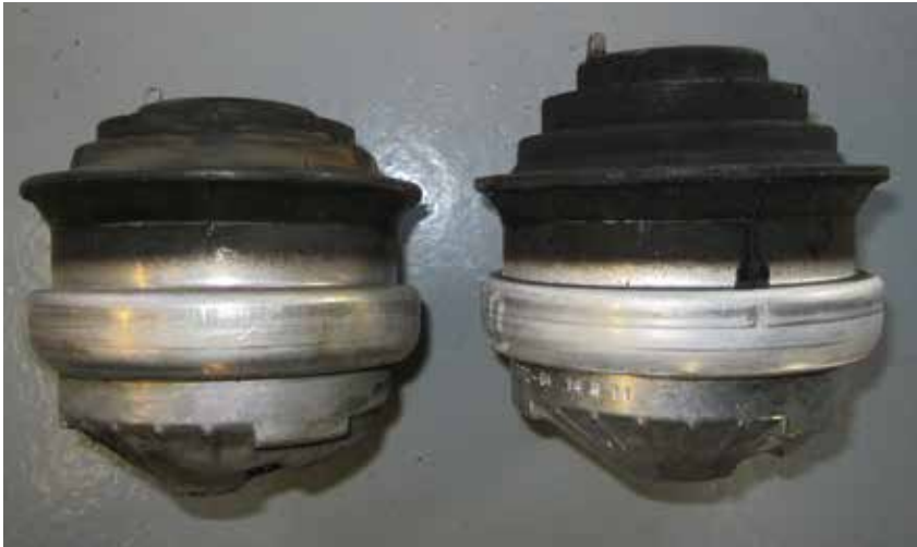
The worn and broken engine mount on the left was causing drive train vibration at all speeds. Notice the height difference to the new one on the right. Installing new mounts restored the vehicle's driveline angles back to normal.
