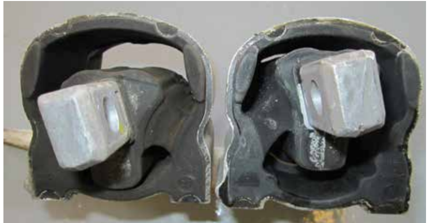
A shot of Mercedes Transmission mounts side by side. The transmission mount on the left is old and collapsed, which caused a driveshaft vibration under acceleration. The right one is the new transmission mount to be installed.
