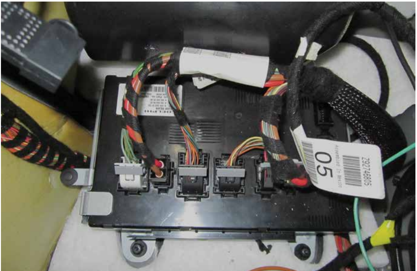
Rear SAM located in the lower rear well of a 2007 GL450.
