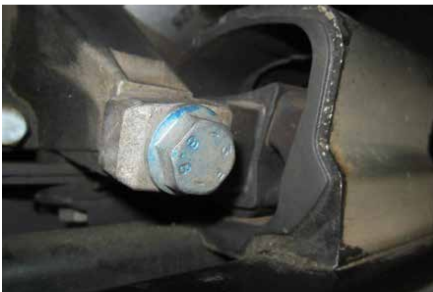
A collapsed transmission mount still in the car. This 2007 E320 had driveline vibration above 40 mph.
