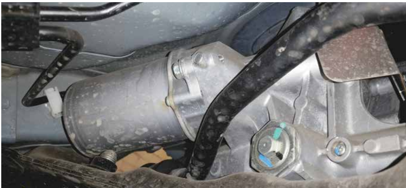
An EPS motor is often mounted directly to the power steering rack, but it can also be mounted to the steering column.
