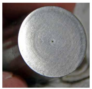
The tiny EDM hole you see is there to promote oiling between the lobe and lifter foot and slow lobe wear when running valve spring pressures that are right up near the high limit for solid lifters. Once you get to about 450 psi over the nose, you can expect to see failures. Extra oil helps.
