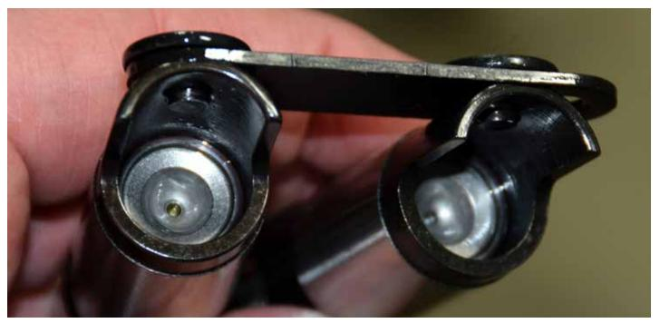
As you can see with this set of Comp solid rollers, there is a huge difference in pushrod seat height between this set and the Jesel. The Jesel lifter seat height is only about 1.190 in. as measured from the bottom of the wheel to the lowest part of the seat pocket. The Comps measure 2.150 in. — almost an inch higher. While this helps by giving us a shorter pushrod, it hurts because of angularity and lifter bore bushing wear.
