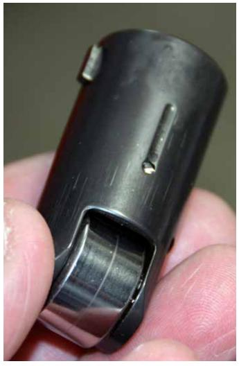
This is an example of some of Dan Jesel's work. This has a "diamond-like coating" (DLC) and is a keyed, low-seat roller lifter. It came out of an SB2 that had an unfortunate accident involving a piece of track debris that snapped the dry sump drive belt at 9,000 RPM. I guess that's why it's called "racing" and not "winning."
