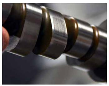
This roller cam has a larger base circle and the lobes don't have inversion ramps. You can still see the pressure mark where the lifter wheel intersected the lobe. These forces actually cause a deformation of the parts involved with stress induced just below the surface of the lobe and roller wheel. Over time, these stresses can lead to cam lobe failures. Good lubrication and micropolishing help.
