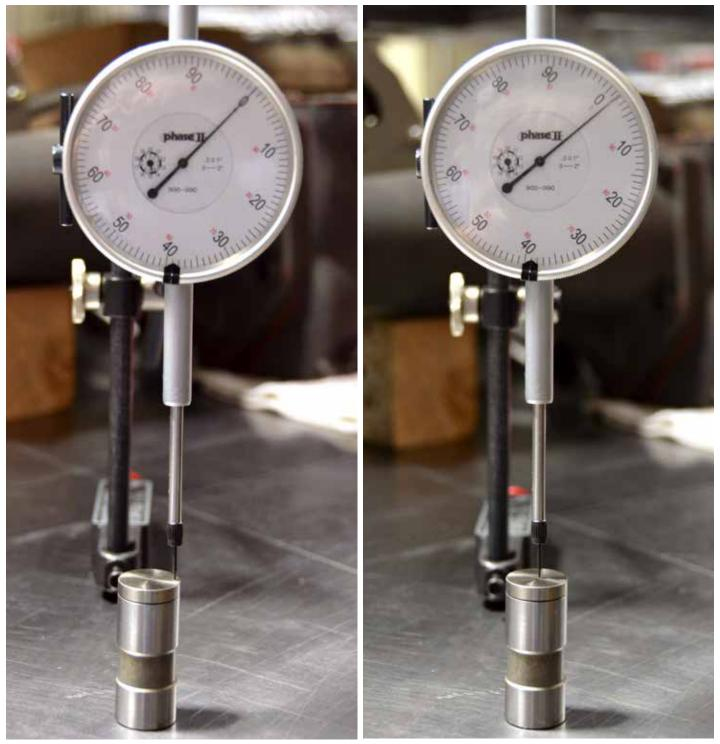
I set the lifter and dial indicator up on a surface plate and measured the difference between the height at the crown and at the edge of the lifter. It measures right at .0018 of an inch.
