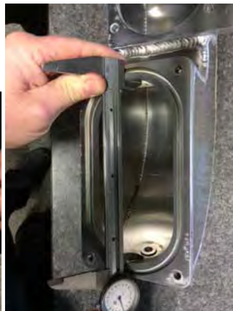
Note that even the welds within a JLP plenum are contoured to minimize restriction to air flow. It's this kind of attention that puts JLP and Kenne Bell products at the top of the charts.
