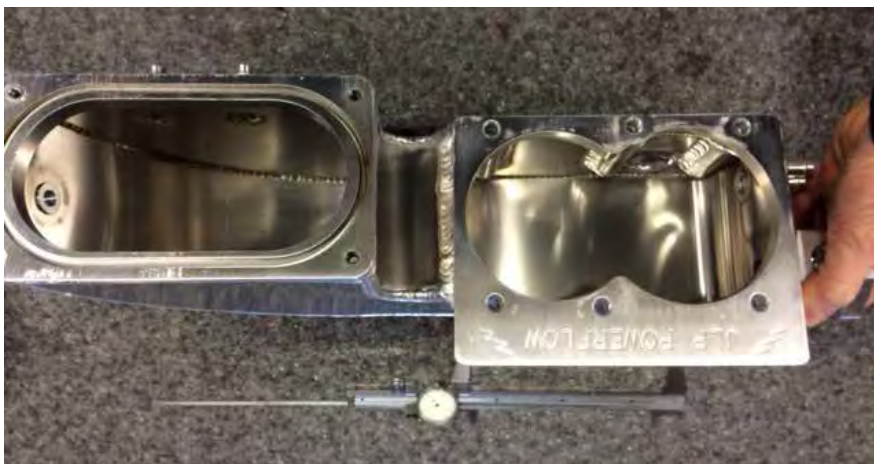
Note that even the welds within a JLP plenum are contoured to minimize restriction to air flow. It's this kind of attention that puts JLP and Kenne Bell products at the top of the charts.
