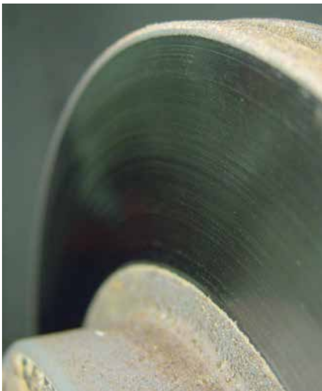
This is typical wear and scoring on a well-used BMW disc brake rotor. While it may not appear severe, it might just put the rotor beyond allowable specs.
