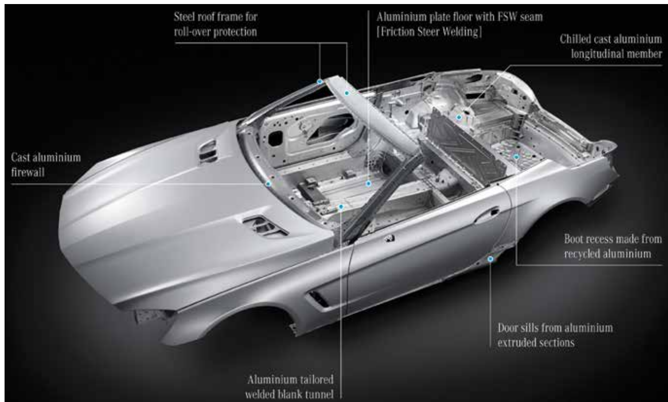
With the exception of the A-Pillar, the 2013 (and newer) SL500 bodyshell is all-aluminum.
