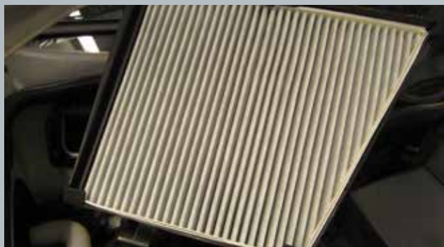
Proper installation of a quality filter. Note the nice seal along all sides that ensures maximum performance.
