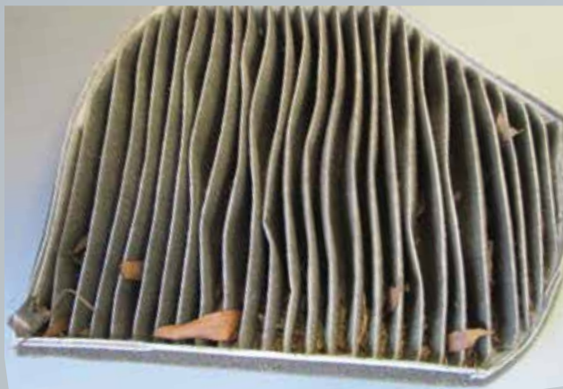
A flimsy, poorly-made cabin filter.
