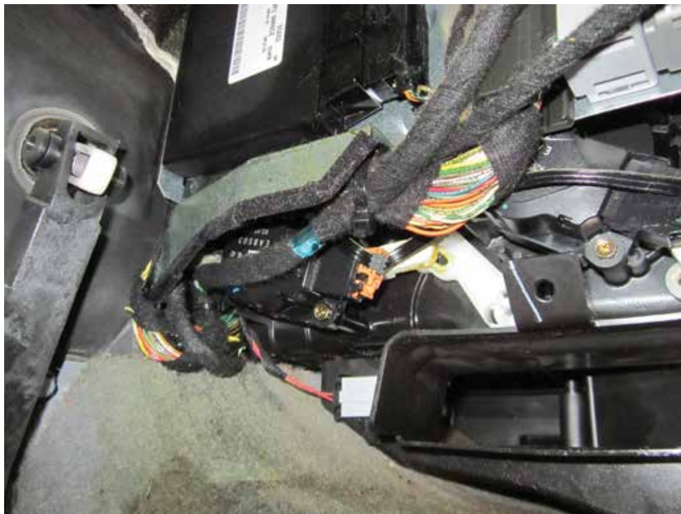
In this under-dash shot of a 2004 ML500 W163, if you look closely you can see where transmission fluid wicked all the way through the harness to the transmission controller above. The ATF then spilled out and contaminated the HVAC stepper motors directly underneath. The initial customer complaint was erratic vent operation.
