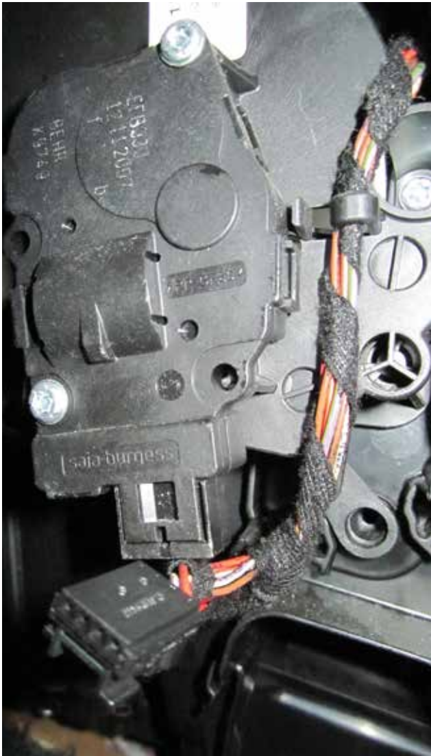
With this LIN system stepper motor, there are no color-coded plugs since these actuators are given a digital address.
