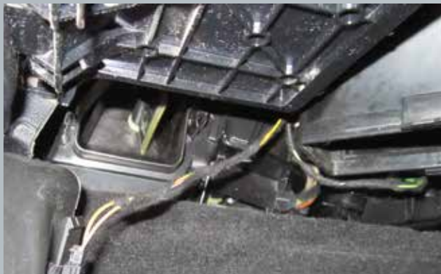
When removing panels to access a cabin filter, care must be taken not to damage components such as this temperature sensor and cable attached to the access panel.
