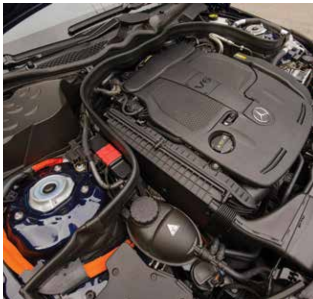
The 2014 E400 Hybrid Sedan crams a 3.5L V6 ICE and a 27 horsepower electric motor under the hood.
