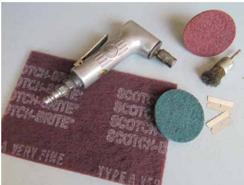
The tools we used to clean sealing surfaces on older engines are way too aggressive for today's engines, and would quickly destroy any chance of proper sealing with an MLS gasket.
