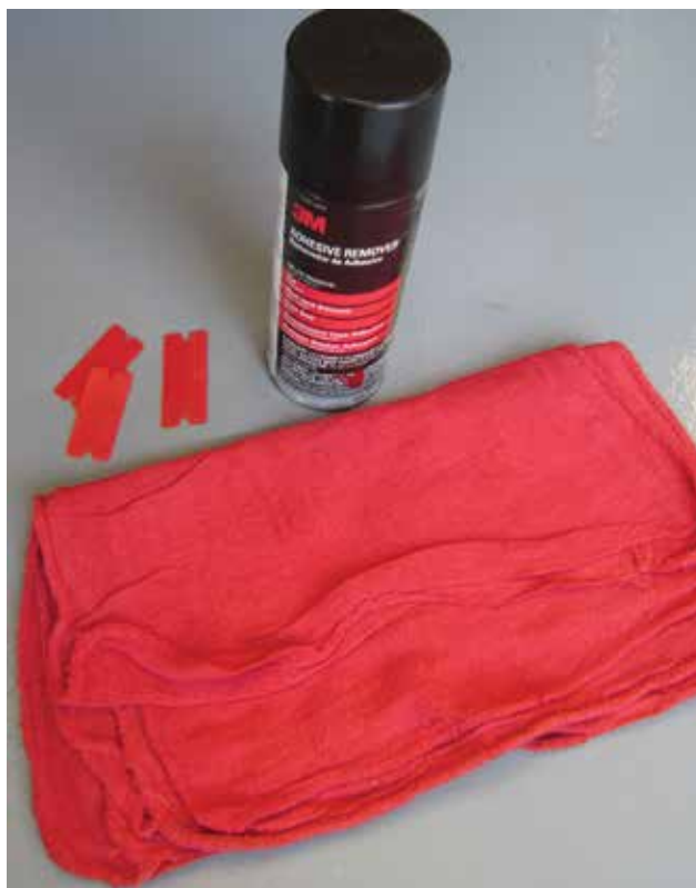
The tools now needed to prep cylinder block deck and head sealing surfaces for the installation of an MLS gasket.
