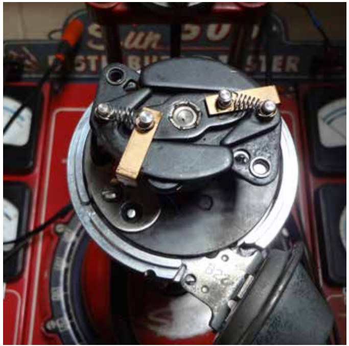
Pertronix Flame Thrower Billet electronic distributors for GM applications come with an assortment of advance stops and springs to allow you to tune the spark advance curve.
