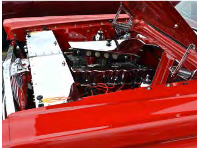
This is the kind of thing that makes it fun. Who would've thought about building a six banger with three carbs on it? Of course, it's a lot nicer to work on than a monster V8 stuffed into that tiny engine bay.
