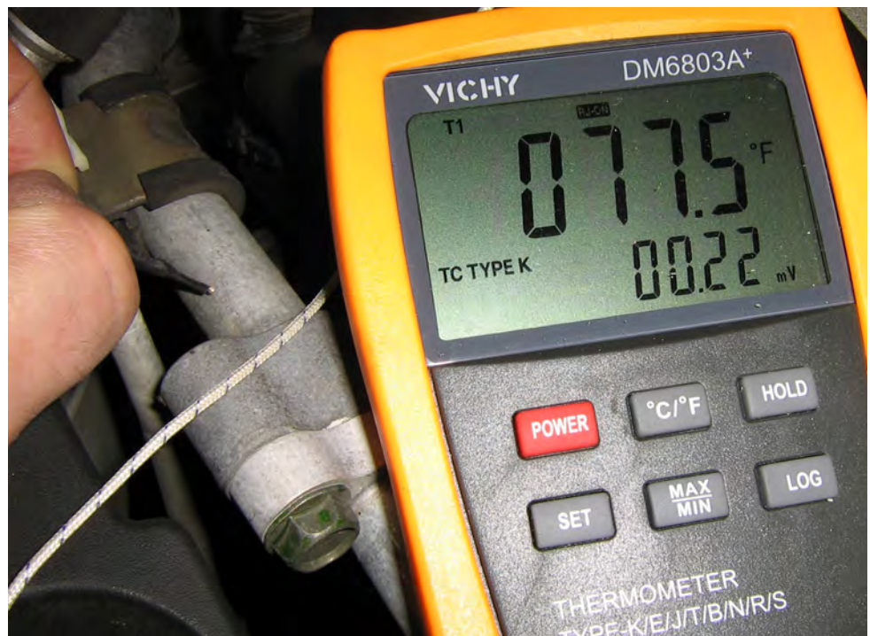
A contact pyrometer is a very useful tool for climate control diagnosis. An infrared thermometer can also be used, but reflective metallic surfaces or attempting to measure small areas can lead to inaccurate readings.
