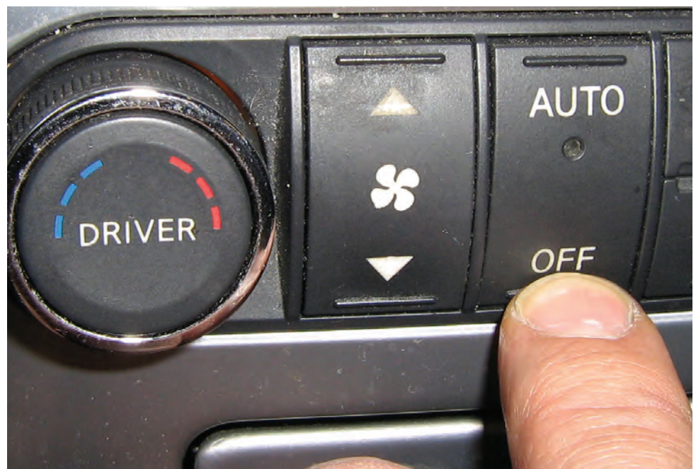
Press and hold the OFF button for five seconds right after starting the engine to enter self-diagnostic mode.
