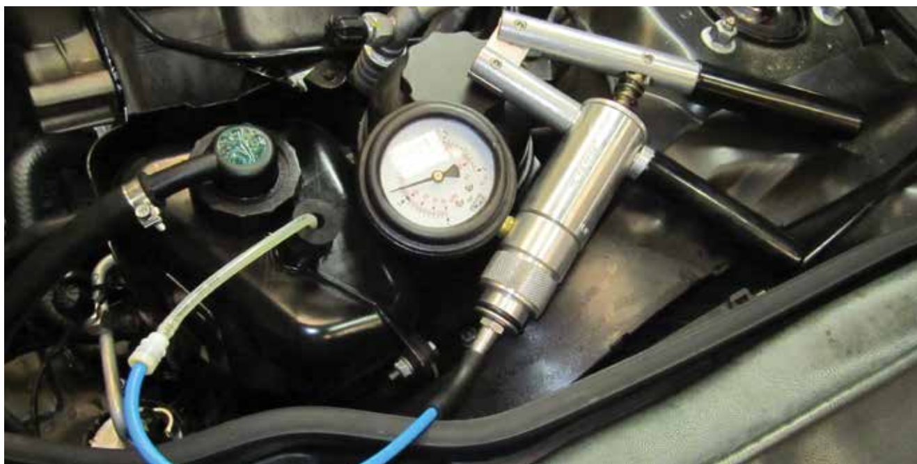
The ABC fluid reservoir must be pre-pressurized to prime a new pump before startup. Failure to do so will dramatically shorten the new part's life.
