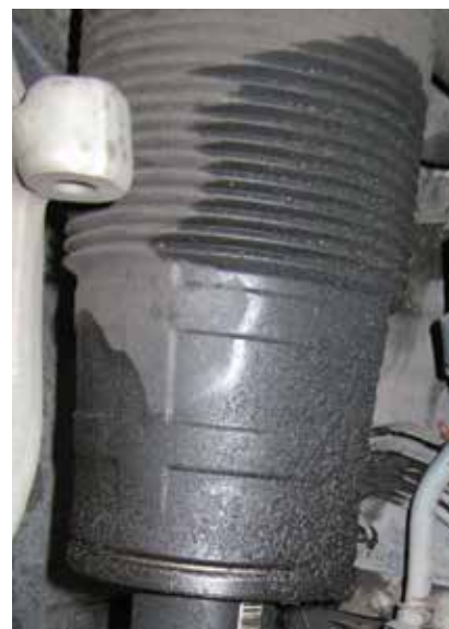
Remember, if fluid can get out, dirt can get in. This heavy leak had been neglected and led to pump replacement along with the shock repair, an expensive proposition.
