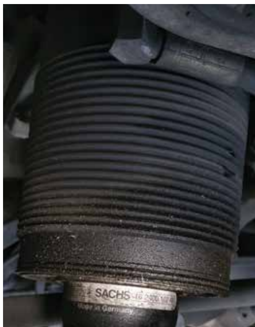
On the rear ABC shock unit, a small leak such as this caught in time can greatly reduce the repair bill.
