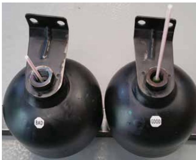
On the left is a ruptured accumulator. Compared to the good one on the right, you can see the difference in straw lengths
