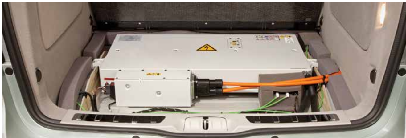
The F-CELL places the high-voltage battery in the trunk floor. The Mercedes-Benz fuel cell system features modular assembly that allows installation in various vehicle configurations.
