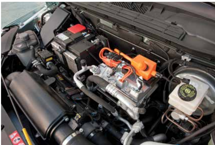
The 2011 Mercedes-Benz B-Class F-CELL packs a power control unit and a fuel cell cooling system underhood where the gasoline engine would be on a traditional ICE (Internal Combustion Engine) powered vehicle.
