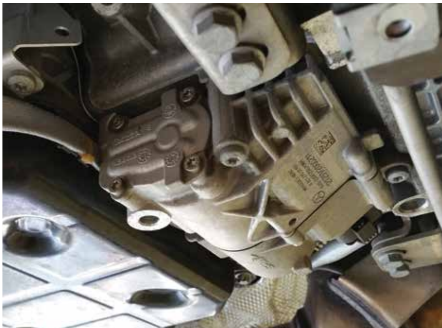
The electric transmission fluid pump maintains positive pressure to keep the transmission ready for rapid resumption of travel.
