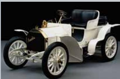
The Simplex had a 5.3L four-cylinder, and could hit 47 mph.
