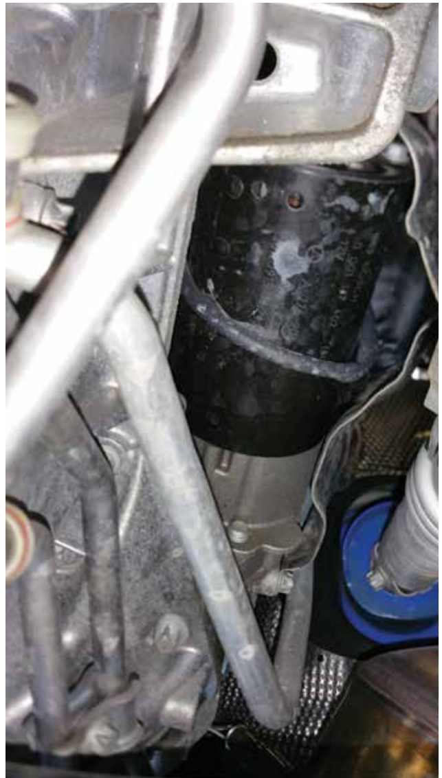
From the outside, an enhanced ECO Start starter looks the same as a normal starter. This makes it imperative that a replacement unit be looked up in EPC and ordered from your local Mercedes-Benz dealer's parts department by VIN.
