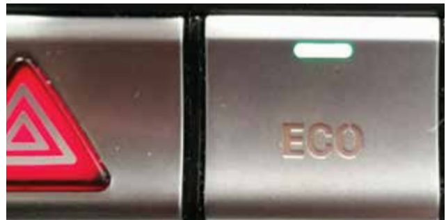
The ECO Start dash button is the only real input the driver can have -- you can turn the system off.
