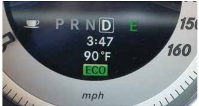
When the ECO Start icon is green, the system is fully functional.
