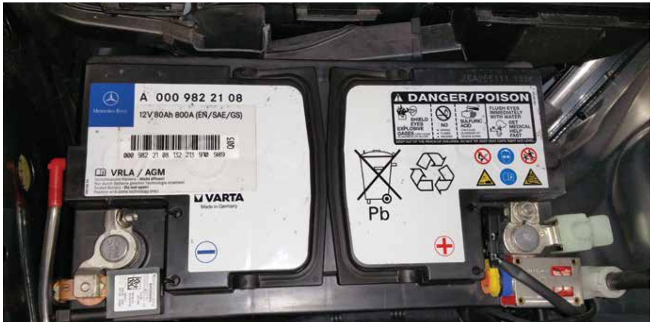
This Mercedes-Benz AGM (Absorbed Glass Mat) battery is an example of the technology that makes ECO Start possible. AGMs can recover from repeated cycling many times more than conventional wet cell batteries can.
