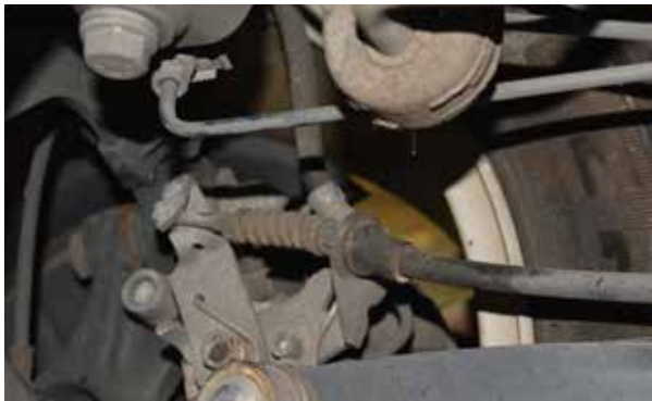
The brake hose, steel line, parking brake mechanism, and other braking system hardware are all close enough to be vulnerable to a hit to the wheel.
