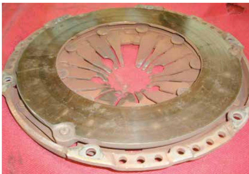
One of the springs on this pressure plate is missing, which is just one of the justifications for always installing a new plate when you're already in there.
