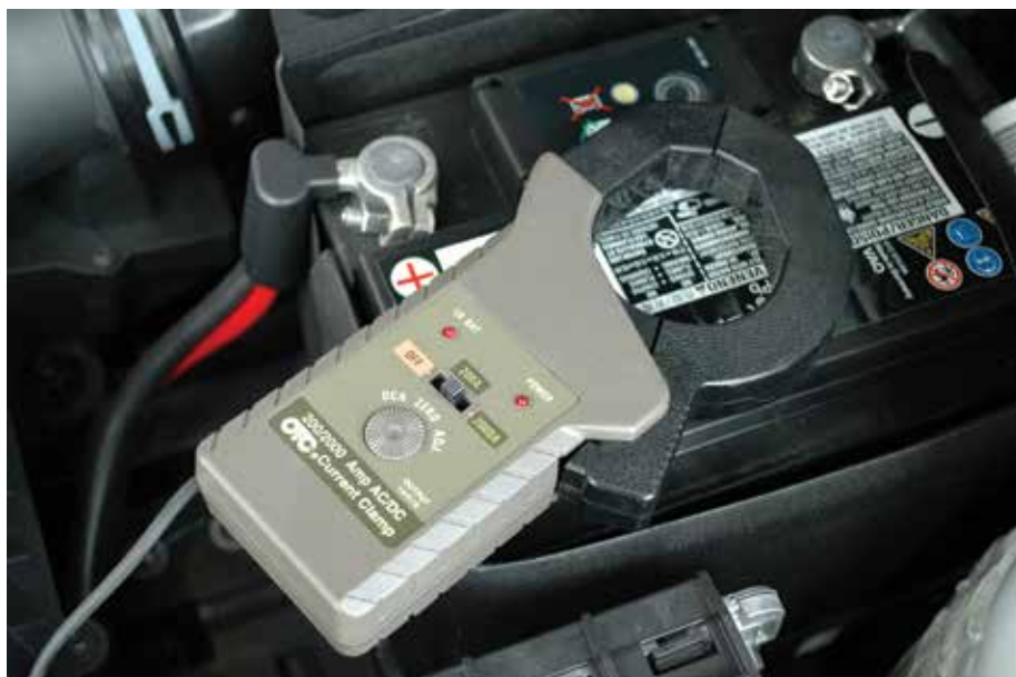
It's much more convenient to use an inductive "amp clamp" than to break the connection and put an ammeter in series.
