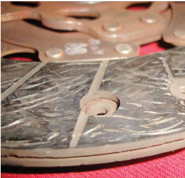
The flywheel side of this clutch disc is just about worn down to the rivets, so it definitely needs to be replaced before the flywheel is gouged.
