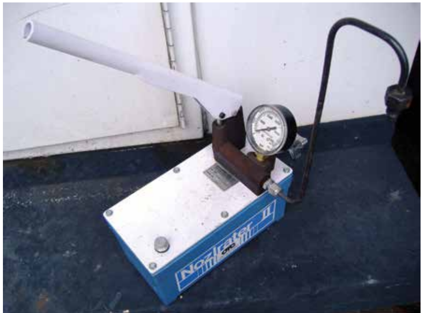
This old pop tester we used for traditional diesel injectors is useless with common-rail. It only goes up to 5,000 psi, which we once thought was a lot.
