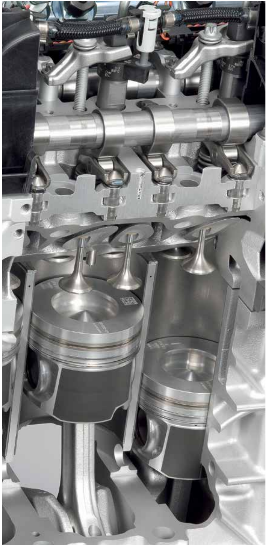
The 2008 six has an aluminum crankcase and coated piston skirts.
