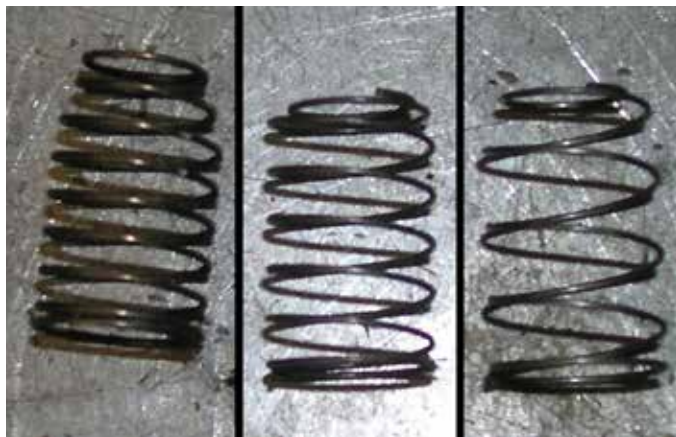
The PCV valve spring on the left is stiffer than the one on the right. The spring rate controls how much vacuum is needed to move the pintle to the low-flow position.
