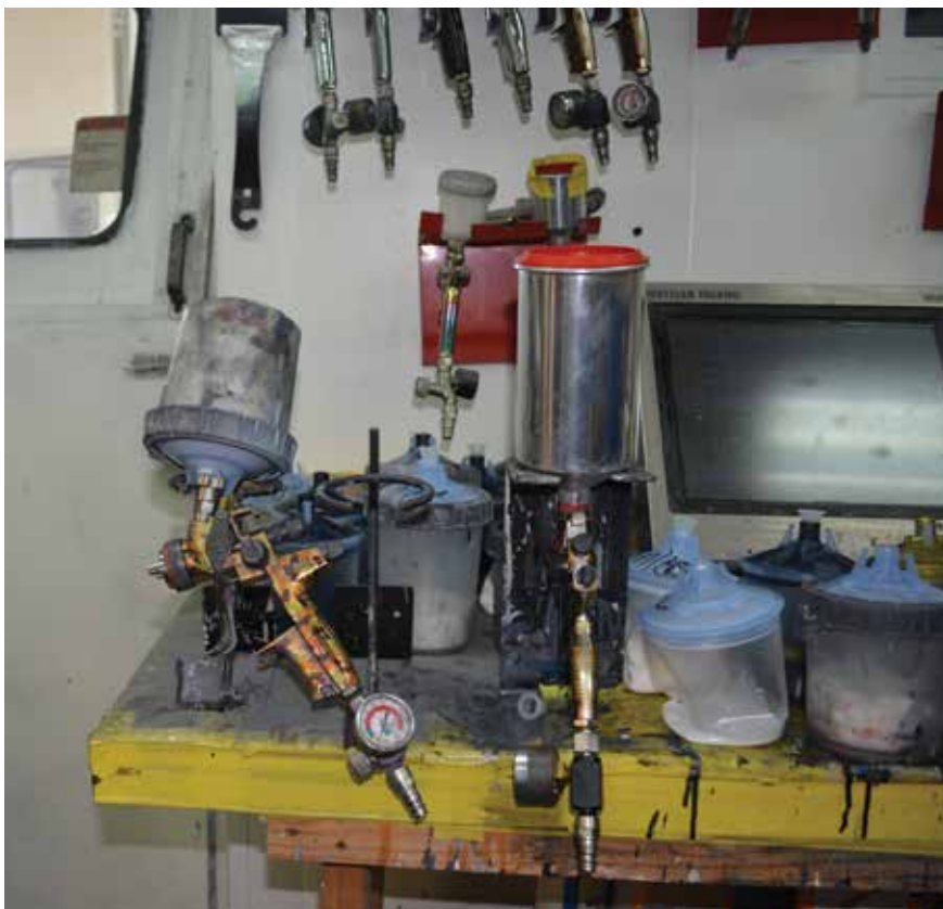
Use separate guns for waterborne basecoat versus clearcoat. Each has a different nozzle size to accommodate the differing viscosities of clear versus basecoat.
