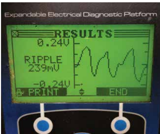
The EXP-800 can be used to quickly test many aspects of charging system performance.
