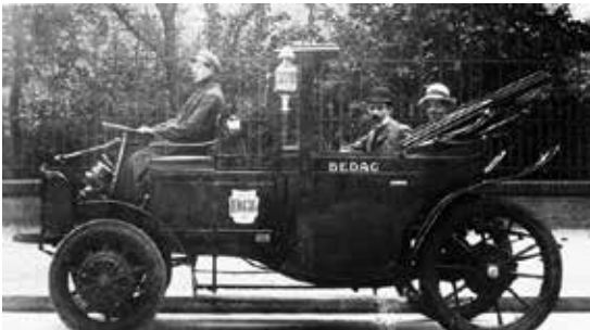
In 1907, the Austrian affiliate of Daimler-Motoren-Gesellschaft introduced the Mixte , a hybrid (Benzine over electric) that saw service mostly as taxis and work vehicles.
