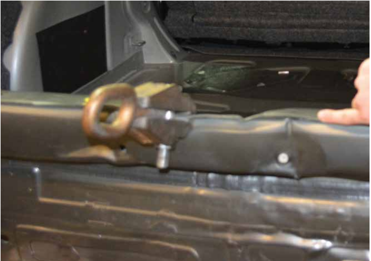
The rear lower body panel on this 2013 VW Tiguan contains HSS, but can be straightened if the damage is minor. Photos courtesy of Jim Ellis Collision Center, a Volkswagen Certified Collision Repair Facility in Atlanta, Georgia.
