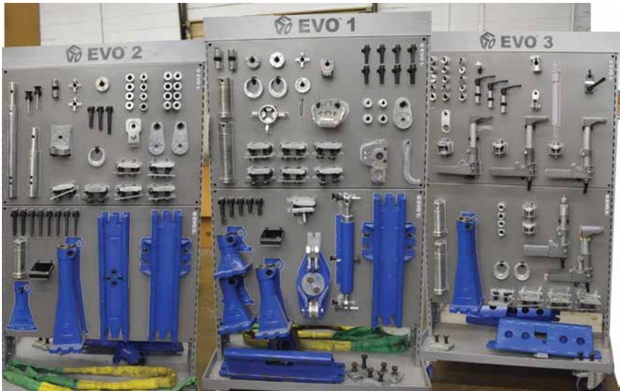
The VW family of anchoring jigs includes basic (EVO 1), specialty (EVO 2), and universal (EVO 3) jig kits that work with any of four different VW-approved Car-O-Liner measuring and alignment systems.
