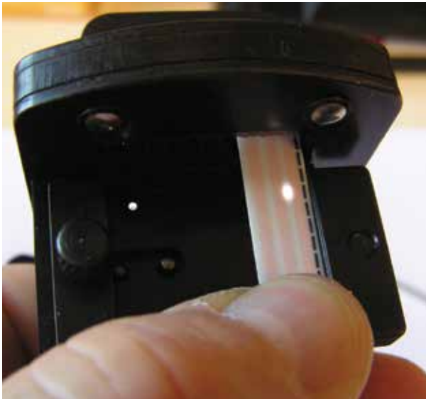
The Mercedes-Benz-approved hand-held crimper for flat cable allows lateral adjustment of the ribbon so that the copper conductors align properly where the cable ends meet. The cable is correctly aligned when light from tiny openings in the tool is fully visible between two conductor tracks.
