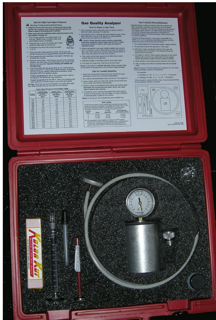
In the field, a Reid pressure tester is used to measure the front-end volatility of gasoline.
