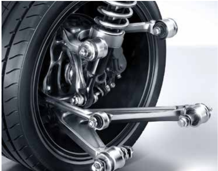
The 2016 AMG GT S uses forged aluminum double wishbones and hub carriers at all four wheels, giving its state-of-the-art Adaptive Suspension system the rigidity needed for excellent road-handling performance while also reducing unsprung weight.
