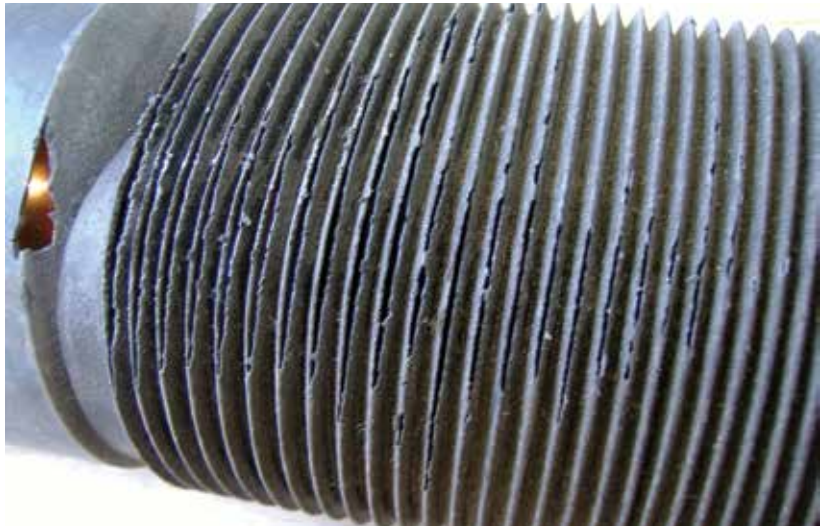
We once saw a tech remove an intake manifold to fix a supposed vacuum leak when the real problem was a perforated duct downstream of the MAF.
