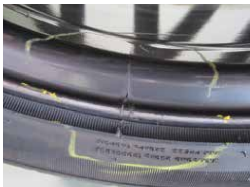
This aftermarket rim is cracked! You're not likely to see that with Mercedes-Benz Original Equipment wheels.
