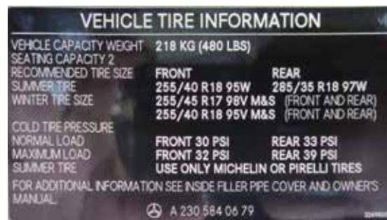
Each vehicle will have its own label indicating acceptable wheel and tire sizes. Of particular note here is the notation that summer tires are of the “staggered” configuration, with larger tires on the rear. However winter tires should be of the same size front and rear.
