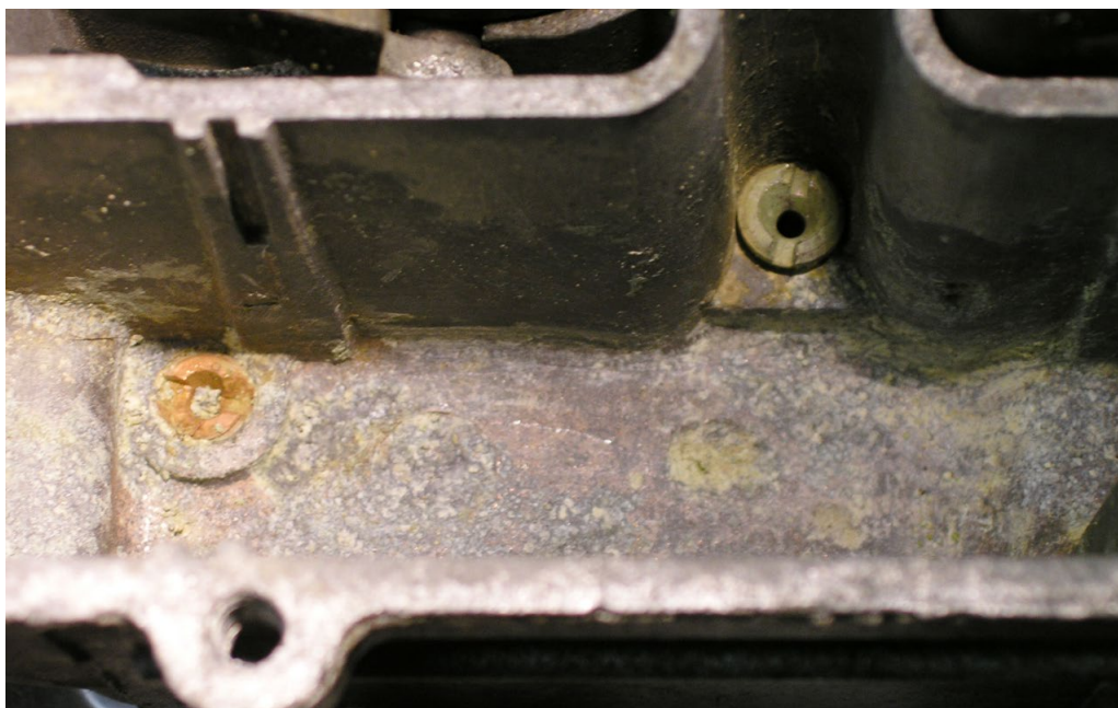
The bottom of this AFB carburetor fuel bowl has been damaged by phase-separated gasoline.
