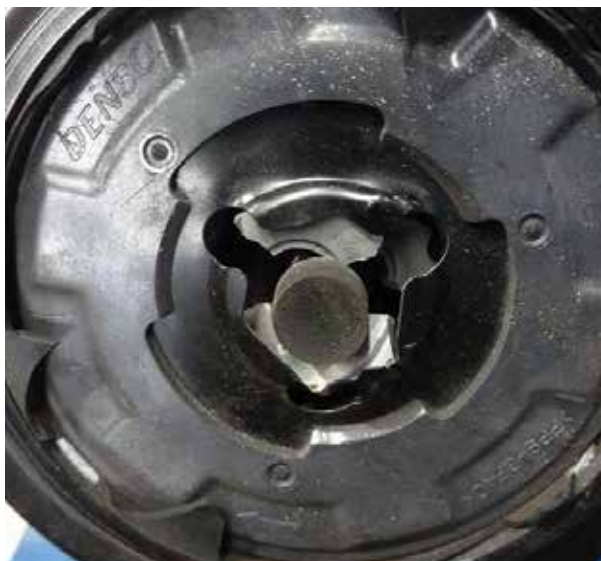
After removing the dust cap, most pulley damage is apparent. This compressor was still spinning, although it was noisy.
