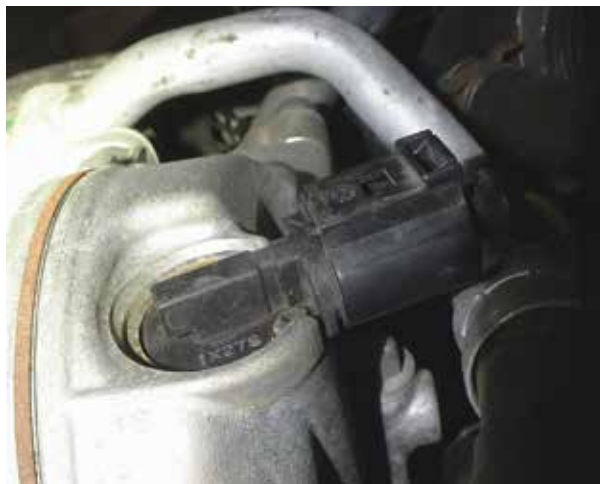
The electrical connector for the regulator valve is accessible from the bottom of the vehicle. A standard two pin connector, it is easy to access for back probing.
