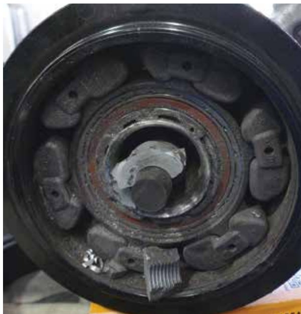
Fully exposed you can see the damage to the compressor.
