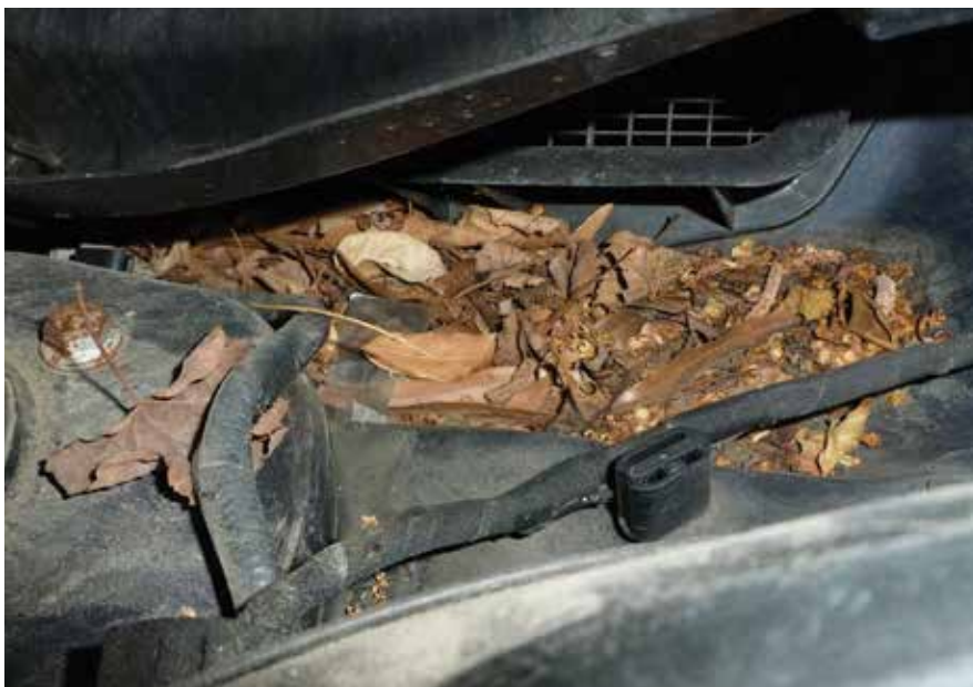
Plant matter tends to accumulate in and around underhood drains. These drains must be periodically cleaned and cleared, just like sunroof drains.
