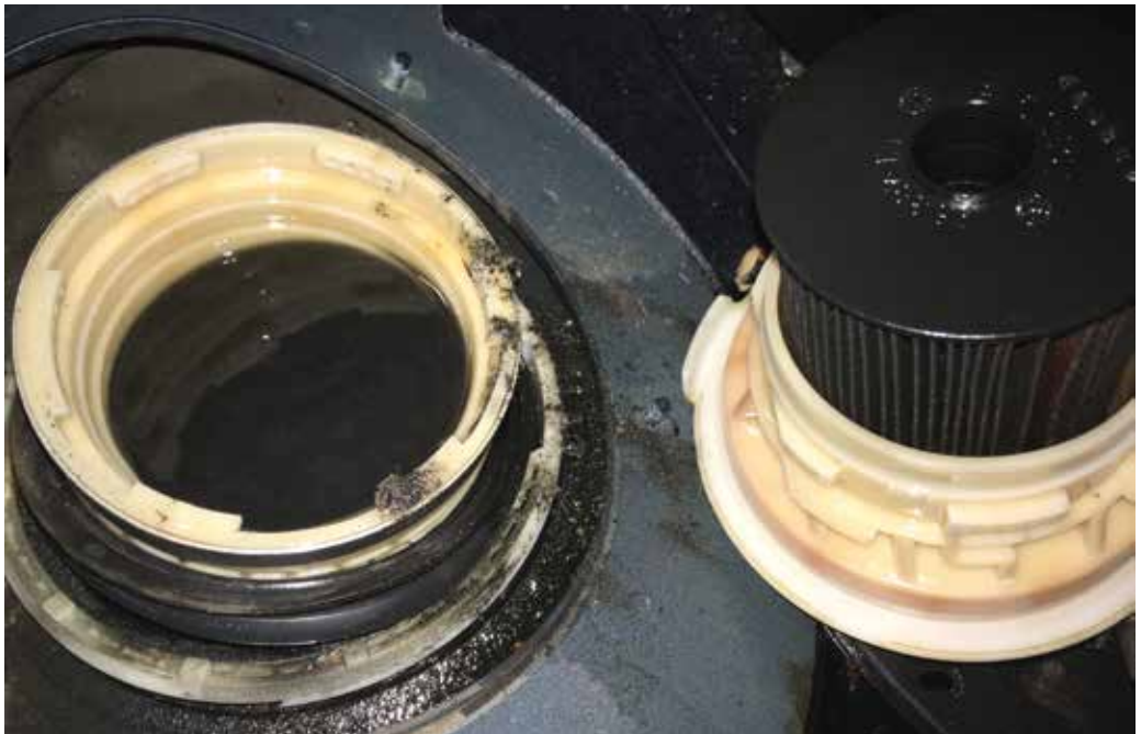
Always replace the fuel filter when replacing a faulty pump. This in-tank filter has become heavily contaminated after less than 120,000 miles of use.
