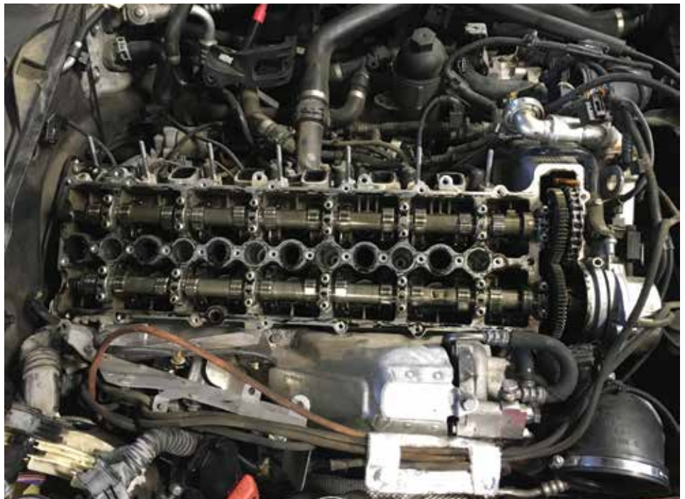
M 57 engine with intake manifold and valve cover removed
