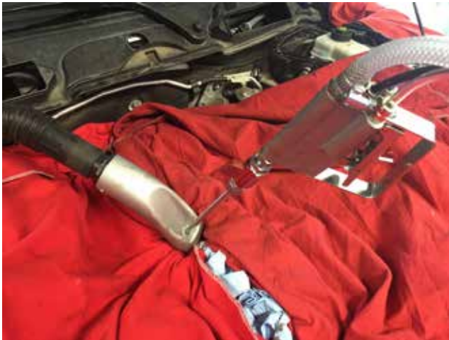
Using carbon blaster on swirl port.
