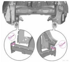
Apply two-part body adhesive (D 180 003 M2) to the side of the bumper bracket facing the rear seat. Fit the replacement floor pan with the vehicle secured to an alignment bracket set on a frame bench, or while it is standing on its wheels.
