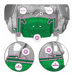
Weld the left and right side front (straight portion) of the floor pan front overlap using MIG/MAG continuous seam welds. Using a MIG/MAG plug weld seam, weld the curved front (1), the vertical reinforcements that drop down to support the spare tire well sides as they curve toward the front, and the sides above the frame rail. Weld the ends of each side using a straight-line spot weld seam.
