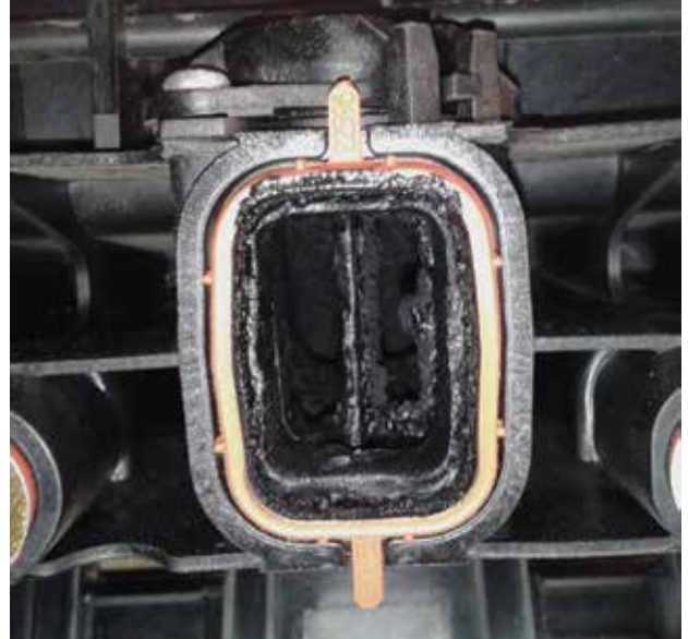
Other places where carbon can build up include the tangential ports on the intake manifold and the tangential ports on the cylinder head.
