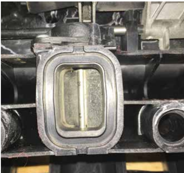
This is a tangential port on an intake manifold with swirl pot closed after soda blasting.
