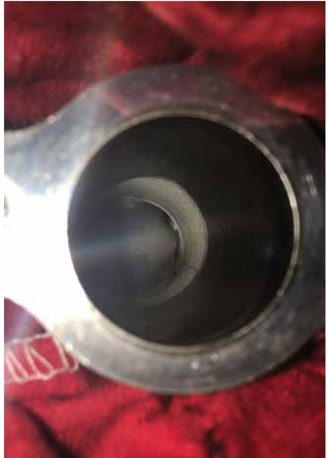
The swirl ports on the cylinder head can look like this after cleaning.
