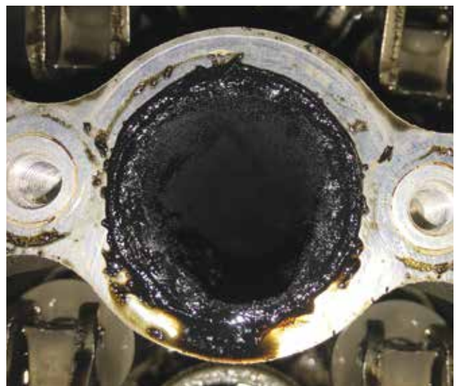
Carbon can build up in cylinder head swirl ports in addition to other places within the induction system.
