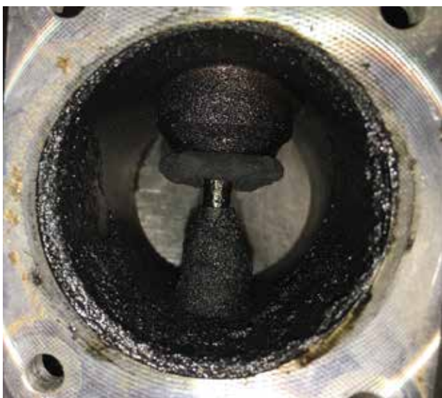
Here you can see how much carbon can develop on the EGR valve mechanism.
