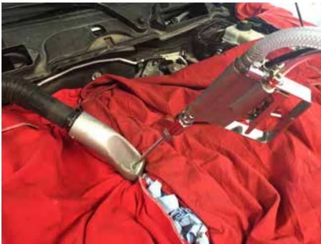
Using carbon blaster on swirl port.
