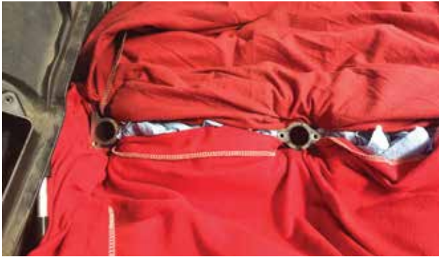
Here is an example of how thoroughly you should seal off ports and passages prior to carbon blasting.
