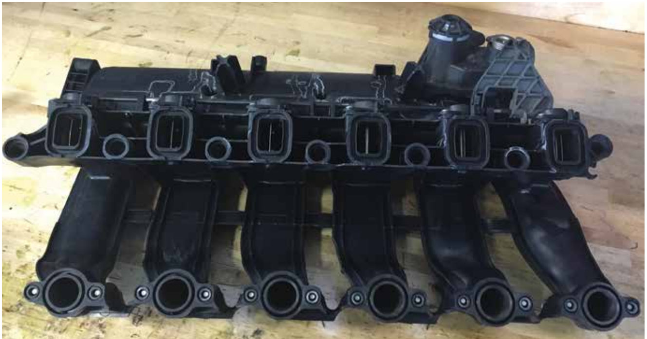
Here is a complete M57 intake manifold reassembled after soda blasting.
