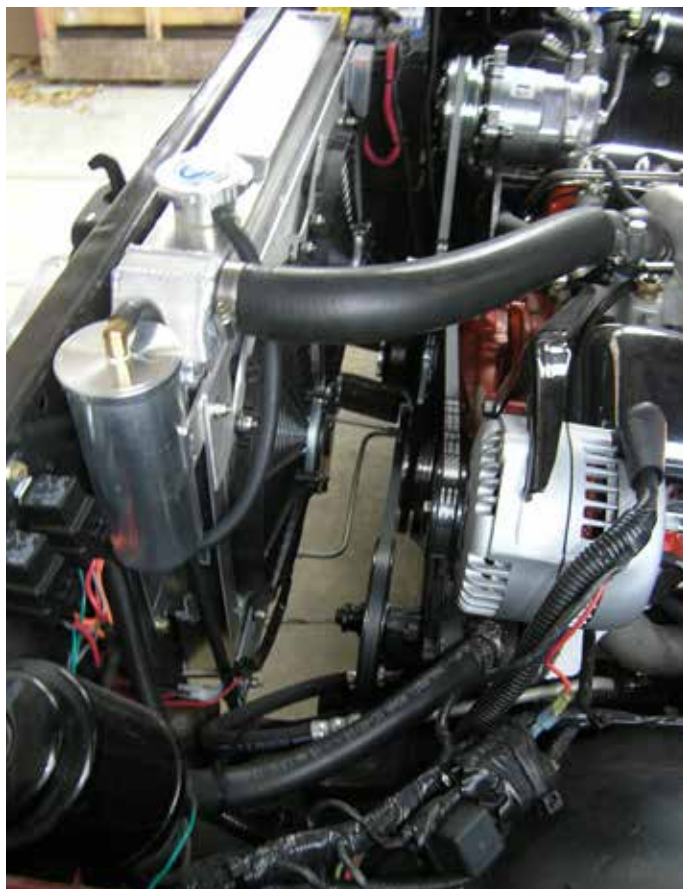
This high-output alternator was not properly aligned to the other pulleys, which caused the fan belt to bend and twist, thus is slipped under load.
