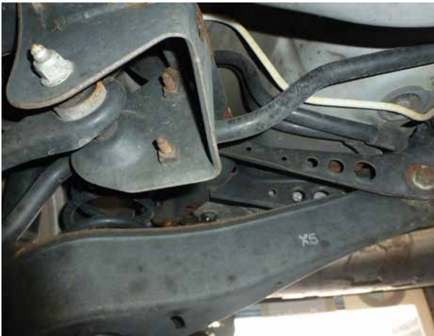
Alignment adjustment points are readily accessible. It's wise to spray bolts with a penetrant to ease movement, particularly in rust-prone areas of the country.
