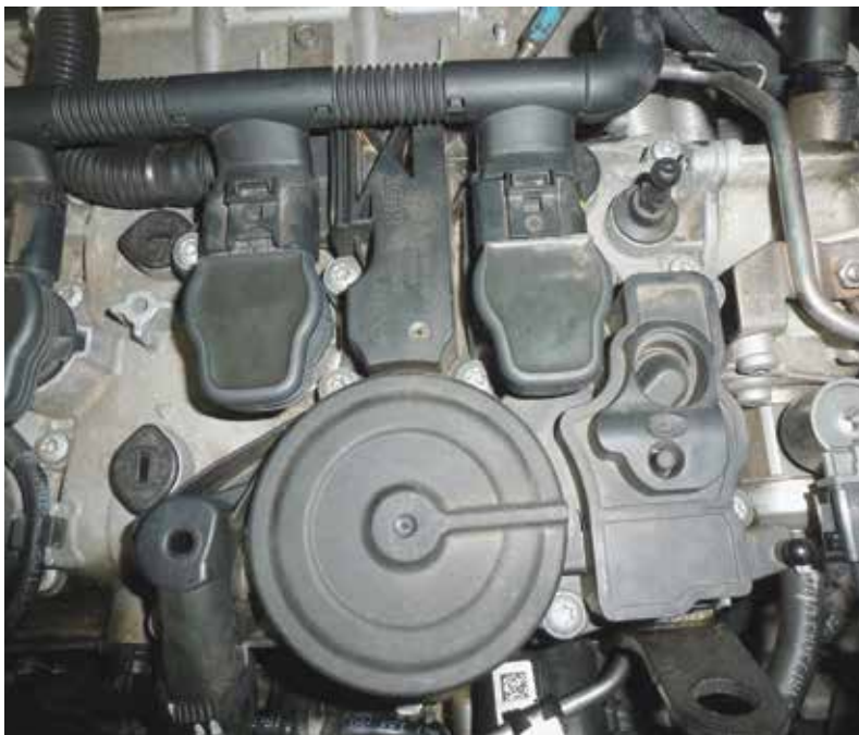
The PCV valve is located directly on top of the cylinder head on the 2.0T engine. It is very easy to replace in event of failure.
