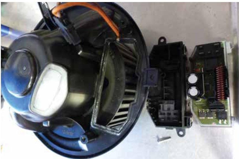
The blower motor resistor is not serviceable. If damaged, it must be replaced.
