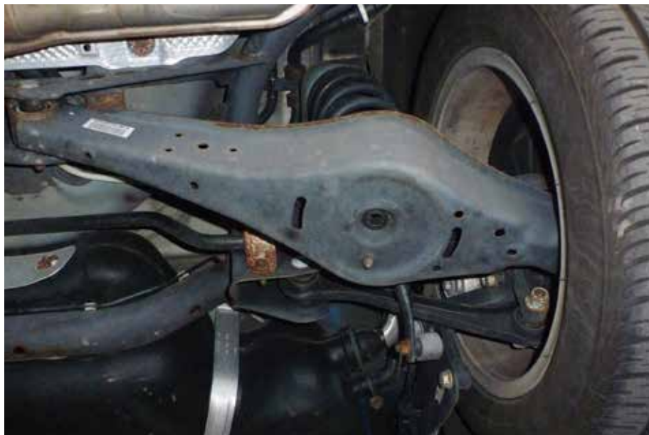
The front lower bushing helps to control and dampen vertical suspension movement.
