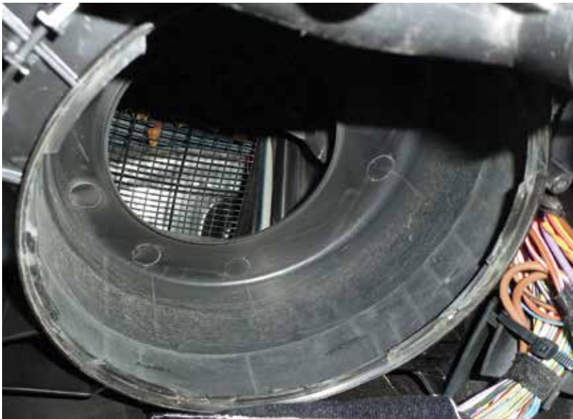
As you can see, the inside of the blower casing is not protected. Any water or material that flows into the intake can fall directly into the blower motor.
