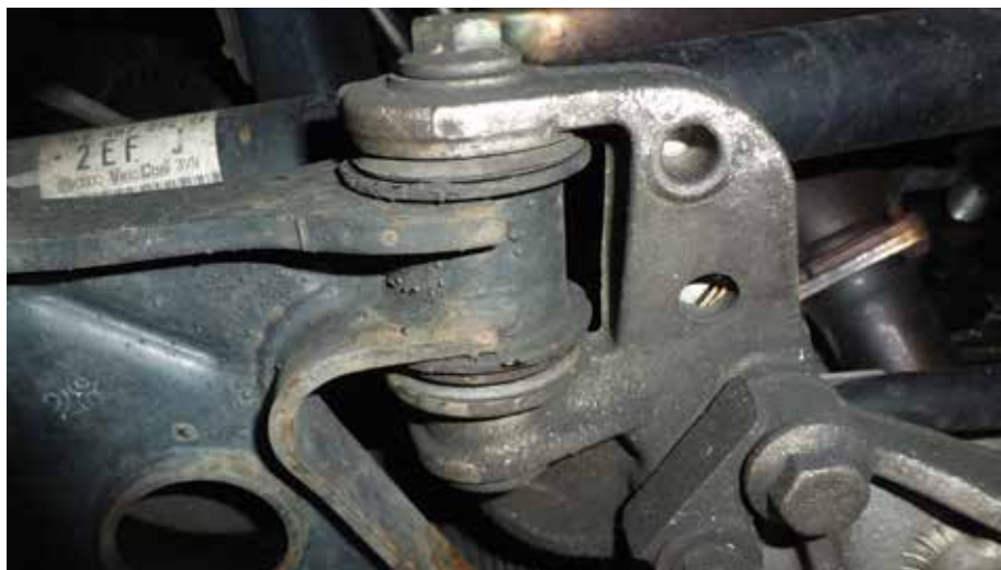
The front lower bushing helps to control and dampen vertical suspension movement.
