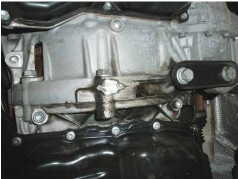
Here is an example of a rear main seal leak. In this case, the leakage has not yet reached the point to cause unmetered air loss. But if left unresolved, it can become a problem.
