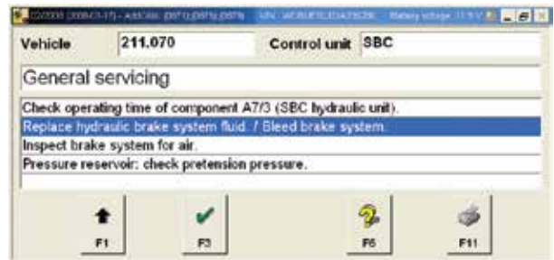
For a couple of decades, a scan tool has been required for proper bleeding and flushing. XENTRY handles the process.
