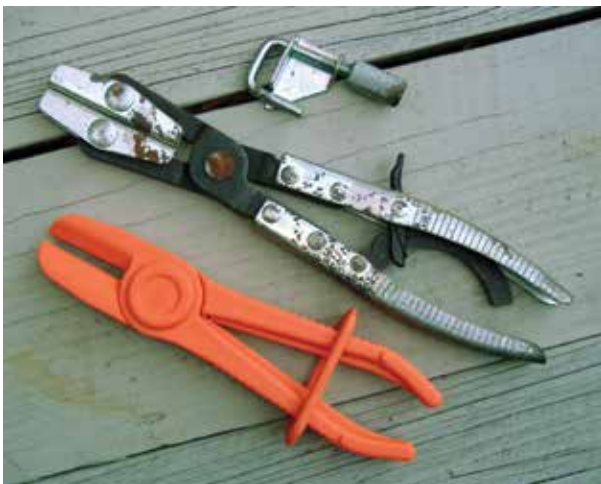
It was once considered smart to isolate wheels using clamps like these. Not anymore. You'll crush the plastic lining.
