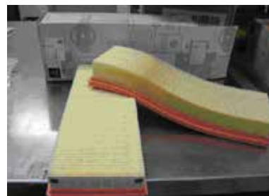
Before you start thinking about replacing a MAF sensor you're dubious about, look into the filter situation. If it's not a genuine Mercedes-Benz part, that could be the whole trouble.
