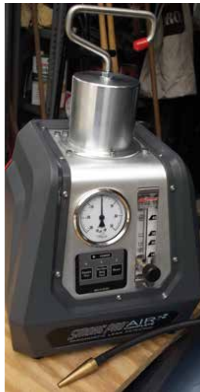
We know of no better way to find elusive intake tract leaks than with a smoke machine.
