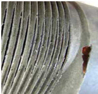
Damage and perforation of the duct between the MAF and the throttle body may have caused many perfectly good sensors to be mistakenly replaced. Better materials and construction are gradually eliminating the problem.
