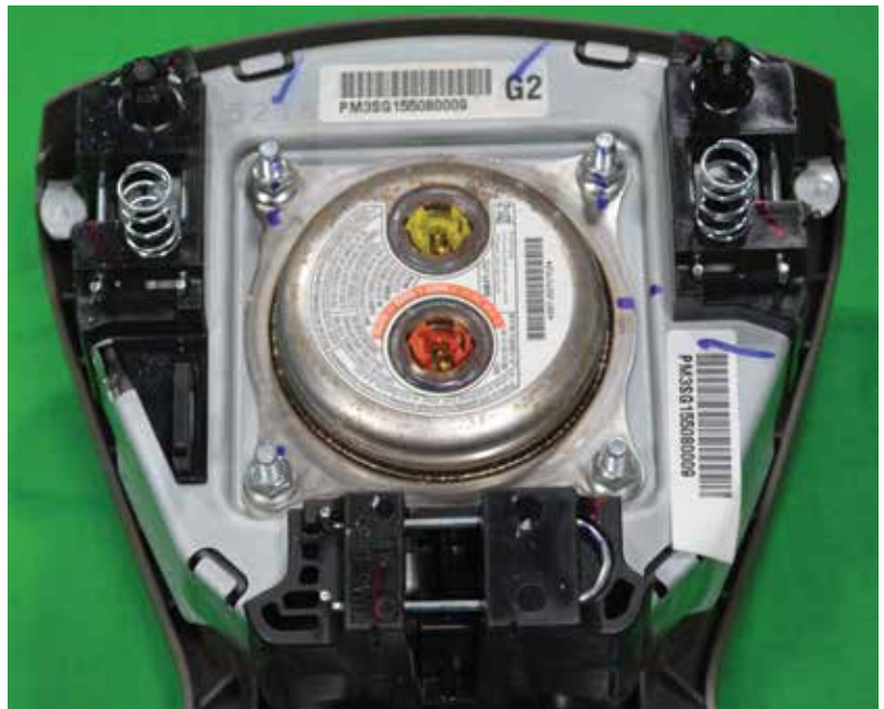
The driver's and front passenger's air bags for most 2007 and newer Nissans are a dual-stage design that includes connections for two separate inflator circuits, one for partial inflation in a minor collision, and a second for maximum inflation in the event of a higher impact. Shown is the driver's air bag for a 2014 Sentra.
