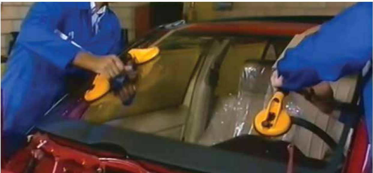
Very carefully align the windshield glass in preparation for installing it.
