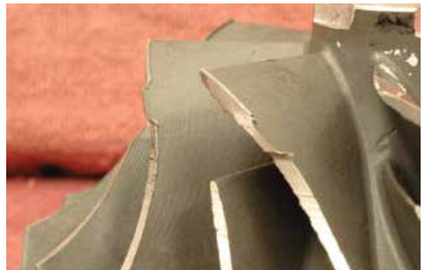
FOD (Foreign Object Damage) only happens if somebody drops a bolt or a socket into the intake.
